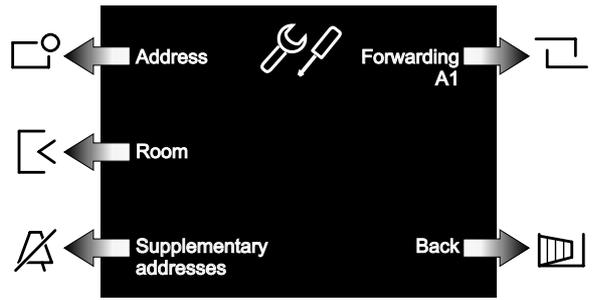
**Address.** Enter the user address corresponding to that memorized in the external stations and the door station. Numbers from 001 to 200.
