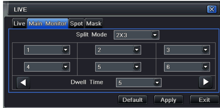
Fig 4-8 live configuration-main monitor
